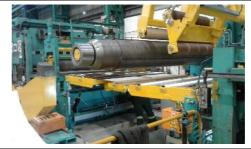
**Fig. 4:** In the recoiling mode, the guide tables are lowered.
