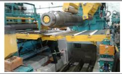
**Fig. 3b:** In the cut-to-length mode, the guide tables are closed, enabling the strip to pass below the recoiler mandrel.
