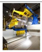
Fig. 2: High-precision bearings of the knife shafts guarantee that GEORG slitting lines provide exact cuts with minimum burr even if a great number of closely arranged cuts are required.
