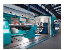
Kreuztal, Germany, August 17, 2016 At AMB GEORG presents the horizontal machining centers of the series ultraturn MC, which processes workpieces up to 250 tons and 4,000 mm diameter. With the successful commissioning of the first machine at Siemens AG in Berlin and installation of two additional machines GEORG is the
