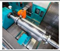
Fig 3: The ultraturn MC at Siemens AG - like all machines of the series - completely encapsulated.
