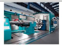
Fig 2: The machining - here the grinding of a generator shaft - and measuring carried out in the same machine.
