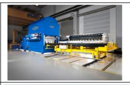
**Picture 2:** The plates run through the line from right to left, at the rear left the stone-type measuring table is located.
