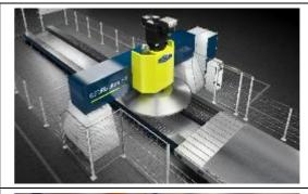
**Fig. 3:** The milling head operates with a drive power of up to 200 kW.
