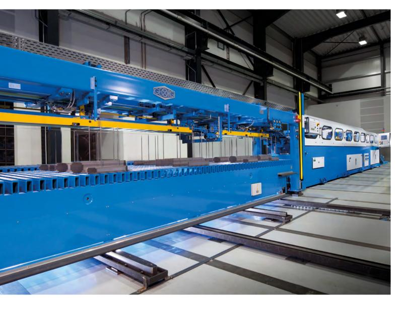
步进铁心片剪切线 **乔格高精确**剪切线TBA400 ecoline L
