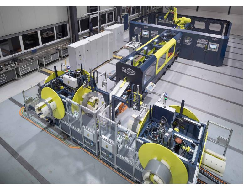
Step Lap Lamination Cutting Line **GEORG precision**cut TBA300 robotline
