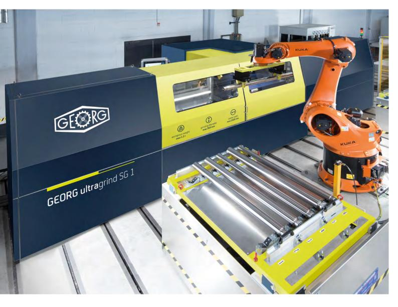
Roll grinding machines **GEORG ultra**grind SG 1
