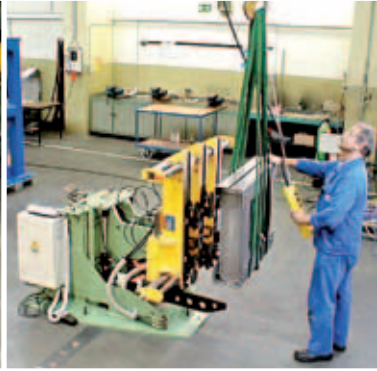
Core removal using crane
